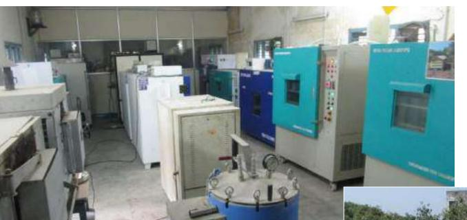
High-temperature, carbonation, humidity chambers
