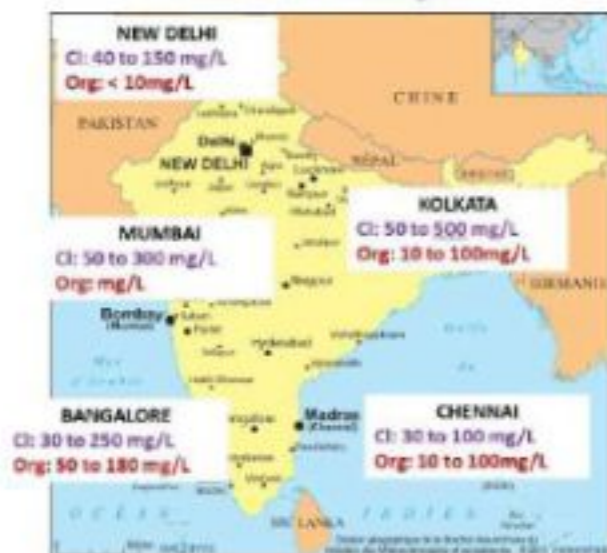
Chloride content of water used for concrete in different regions
