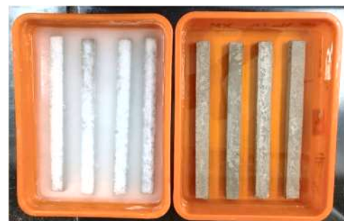
Fig. 5. Photos showing partially carbonated grout specimens immersed in 1 M Ca(OH)_2 (shown on the left) and 1 M Na_2CO_3 (shown on the right) solutions.
