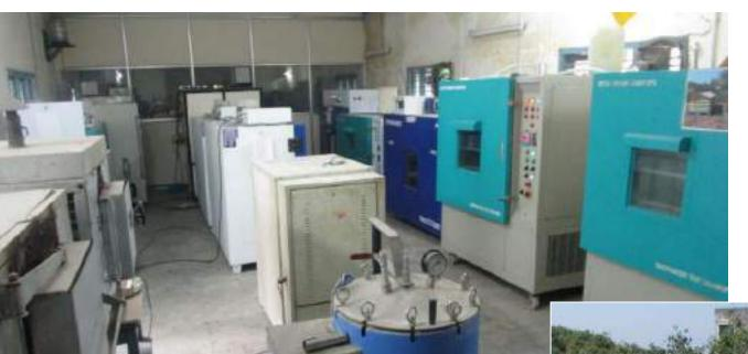
High-temperature, carbonation, humidity chambers
